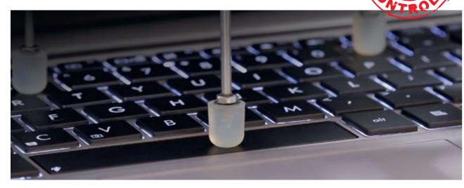
**Keyboard Test** ASUS tests the keyboard to check the comfort and durability, especially on keys that are more frequently used.
